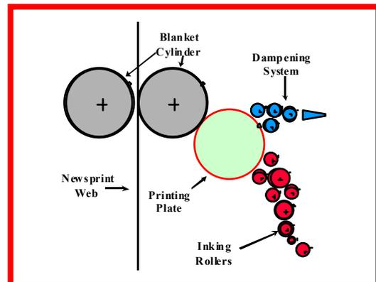
The ink is applied to the printing plate through a series of rollers. These rollers serve to thin the ink film so the proper amount is applied to the plate. The fountain solution can be applied in several different ways: the solution can be sprayed on, transferred from a high-speed brush or by a molleten or sock roller.
