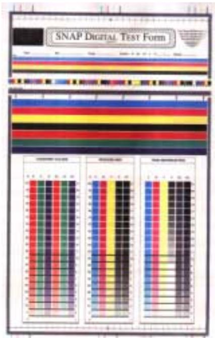
this test run the solid ink densities are set to industry specifications such as SNAP, GATF, NAA.
