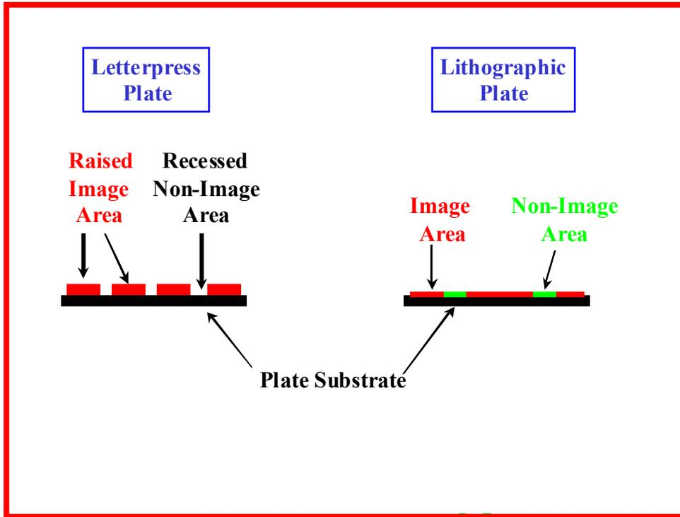
This section is a generalization of the types of printing processes for newspapers. Various manufacturers of printing presses utilize different designs for their presses. The intention of this paper is to give an overview of the processes so that one can contrast the differences.
